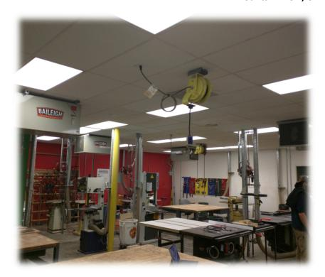
This project involves multiple tool shops within one the Googleplex buildings on Space Park Way. Tool hook-ups were required in the Wood, Machine, Welding, and Electronics shops. Redesigning the existing automated dust collection system was required.
